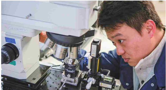
The micro-material testing device, developed at the Advanced Materials Research Lab. This device examines the mechanical properties of minerals.
