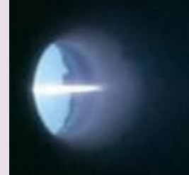
High energy density plasma to radiate EUV (Extremely Ultra Violet) for a next generation Lithography.
